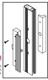
Assemble the Inner and Outer Handles, sandwiching the Lock Stile between them. Tighten the screws just enough to ensure the handle is just secure.
