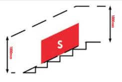
SAFETY GLAZING BETWEEN BROKEN LINES AS MARKED WITH 'S'
